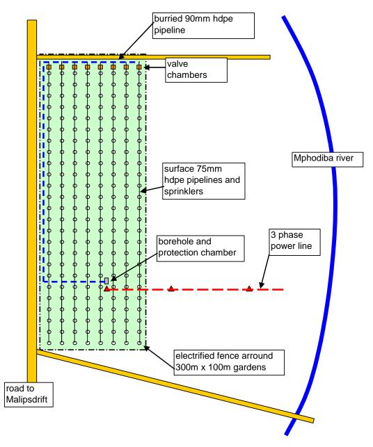
**Figure 3** – Plan of Irrigation system, power supply, and fencing, assuming 3 hectare option
